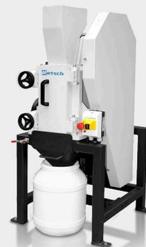
The Jaw Crusher BB 250 is used for the **rapid, effective crushing and pre-crushing of medium-hard, hard, brittle and tough materials**. Its variety of materials offered, including heavy-metal free steel, its efficiency and safety makes this jaw crusher ideal for sample preparation in laboratories and industrial plants.
